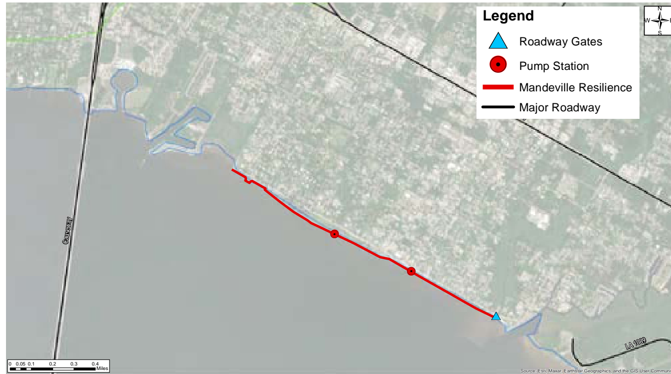
Figure 1-5 City of Mandeville Seawall Alignment
